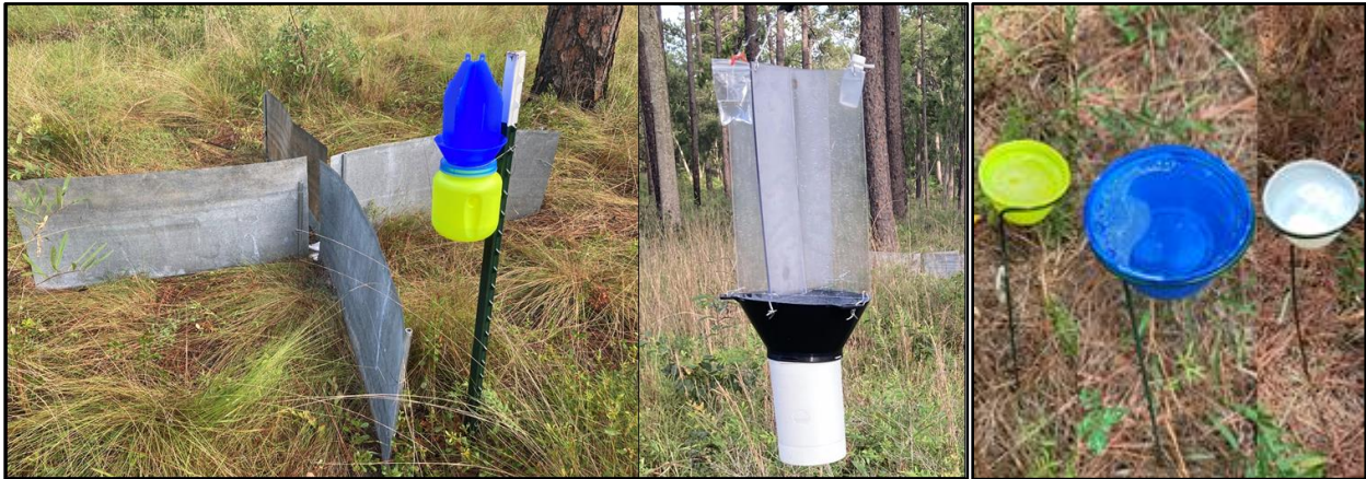
Figure 1. (From L to R) Pitfall trap with barrier, blue vane trap, baited flight intercept trap, bee bowls.
